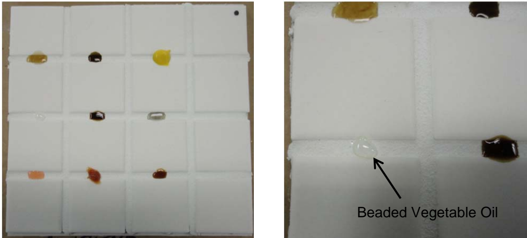
Figure 3. Polyblend Grout prepared with Grout Boost 30 minutes after application of staining agents
