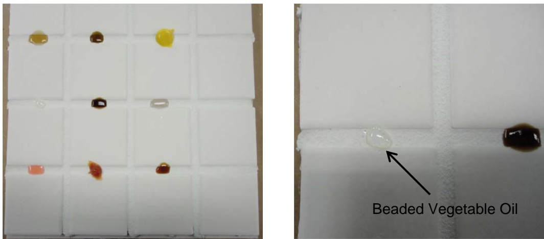
Figure 2. Polyblend Grout prepared with Grout Boost 5 minutes after application of staining agents
