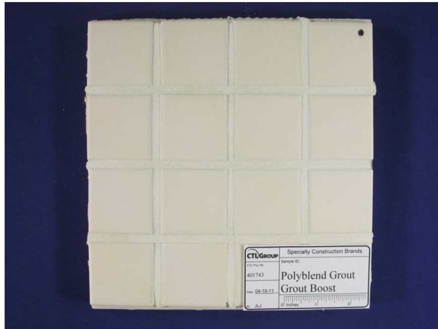
Figure 6. Appearance of tile board prepared with H.B. Fuller Construction Products Inc. Grout Boost 24 hours after removal of staining agents with warm water
