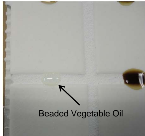
Figure 4. Mapei Keracolor S Grout prepared with Grout Maximizer 5 minutes after application of staining agents
