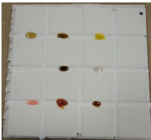
Figure 2. Mapei Keracolor S Grout prepared with Grout Boost 5 minutes after application of staining agents
