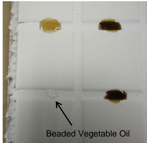
Figure 3. Mapei Keracolor S Grout prepared with Grout Boost 30 minutes after application of staining agents
