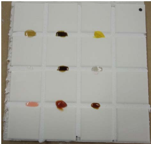
Figure 3. Mapei Keracolor S Grout prepared with Grout Boost 30 minutes after application of staining agents
