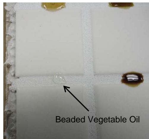
Figure 2. Mapei Keracolor S Grout prepared with Grout Boost 5 minutes after application of staining agents
