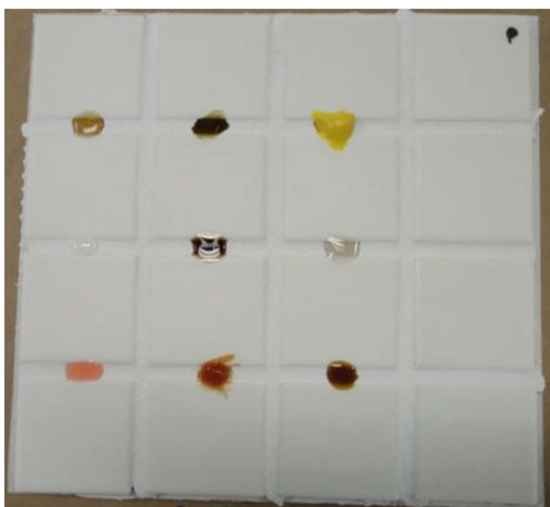
Figure 5. Mapei Keracolor S Grout prepared with Grout Maximizer 30 Minutes after application of staining agents
