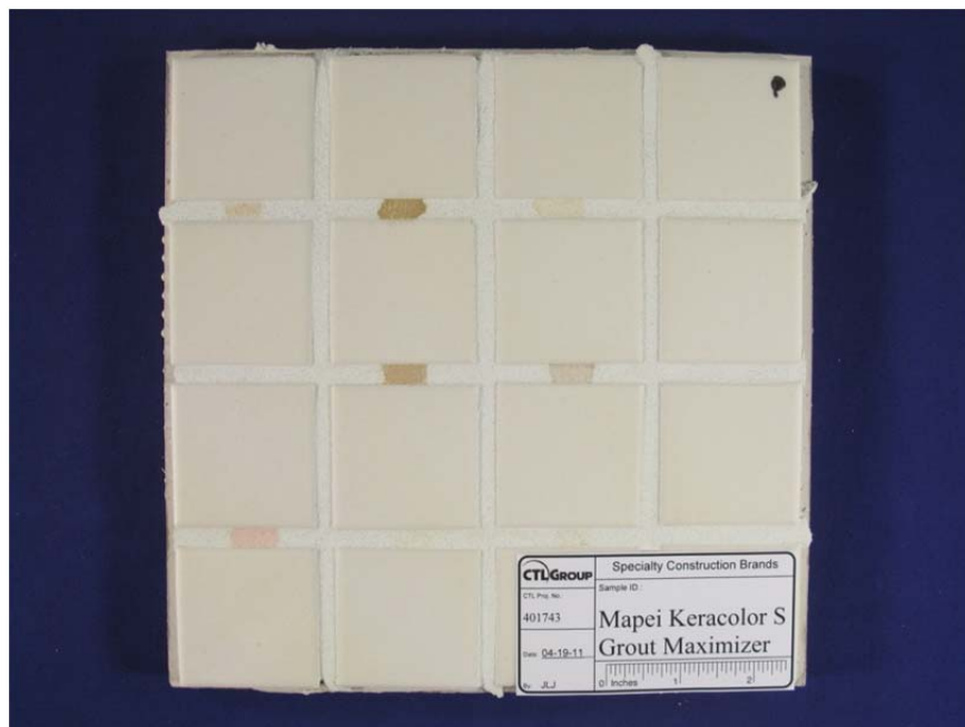
Figure 7. Appearance of tile board prepared with Mapei Grout Maximizer 24 hours after removal of staining agents with warm water
