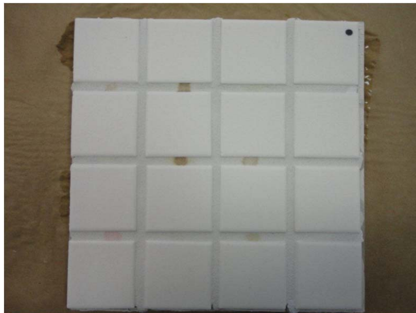
Figure 6. Final appearance of tile board prepared with Miracle Sealants Company Grout Shield after removal of staining agents with Miracle Sealants Company Heavy Duty Acidic Cleaner
