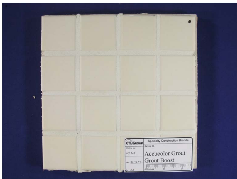
Figure 2. Appearance of tile board prepared with H.B. Fuller Construction Products Inc. Grout Boost 24 hours after removal of staining agents with warm water
