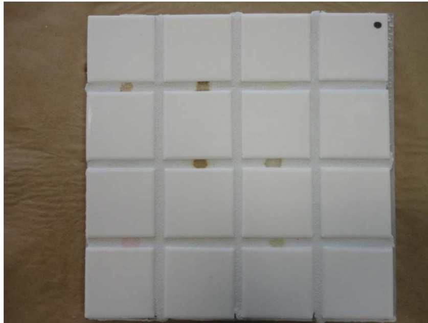
Figure 5. Appearance of tile board prepared with Miracle Sealants Company Grout Shield after removal of staining agents with Miracle Sealants Company Tile & Stone Cleaner
