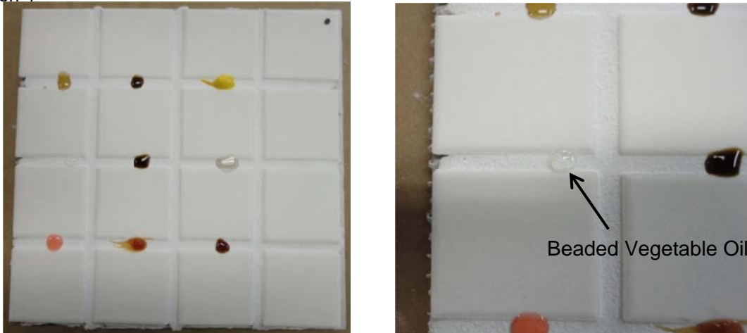
Figure 3. AccuColor Grout prepared with Grout Boost 30 minutes after application of staining agents
