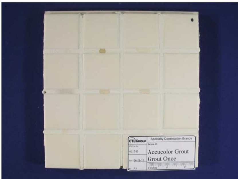
Figure 7. Appearance of tile board prepared with VanHearron Grout Once Improved Formulation 24 hours after removal of staining agents with warm water
