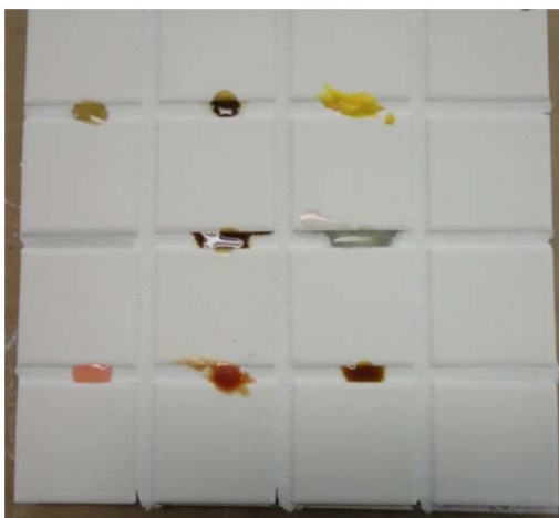
Figure 5. AccuColor Grout prepared with Grout Admix 30 minutes after application of staining agents
