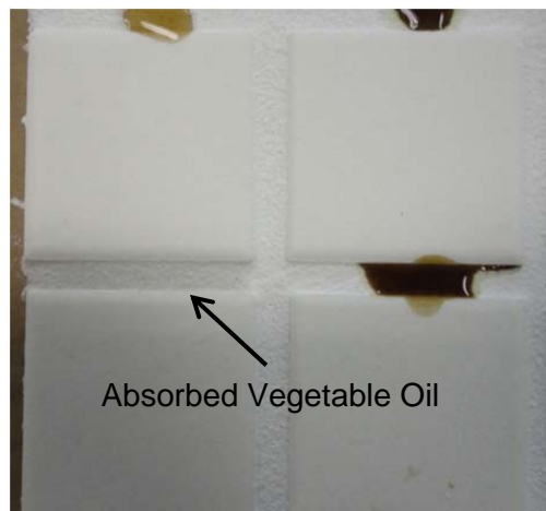
Figure 5. AccuColor Grout prepared with Grout Admix 30 minutes after application of staining agents
