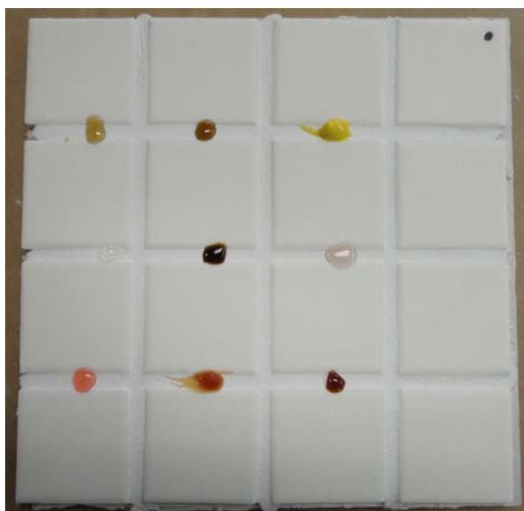
Figure 2. AccuColor Grout prepared with Grout Boost 5 minutes after application of staining agents
