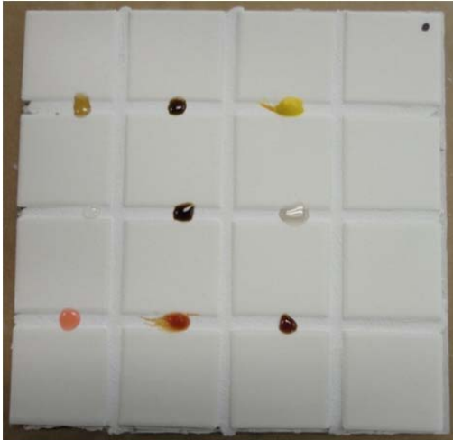
Figure 3. AccuColor Grout prepared with Grout Boost 30 minutes after application of staining agents
