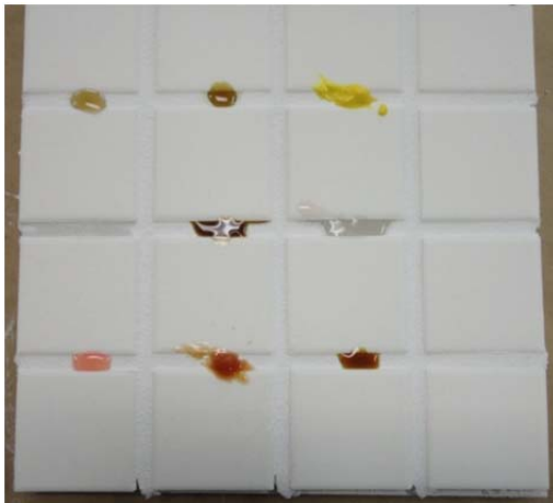
Figure 4. AccuColor Grout prepared with Grout Admix 5 minutes after application of staining agents
