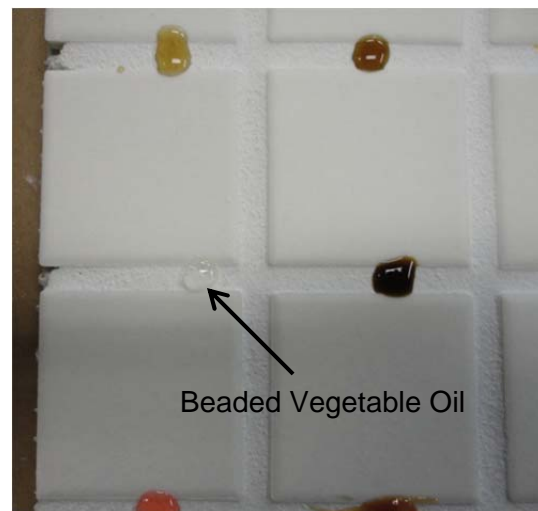
Figure 2. AccuColor Grout prepared with Grout Boost 5 minutes after application of staining agents
